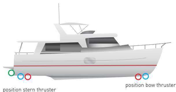
Fig. 7: mounting displacement hull boat
