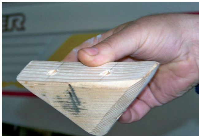
Fig. 24. Contact surface using a wooden wedge as an example
