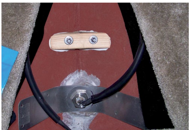
Fig. 25: Screw connection GRP in the boat interior
