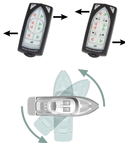
Activating both bow and stern thruster to rotate the boat on axis
