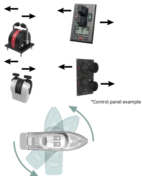
Activating both bow and stern thruster to rotate the boat on axis
